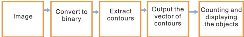
Figure 8.1 Diagram block of the system for calculating number of objects.
