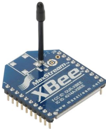
Figure 4.5 Wireless communication using XBee.
