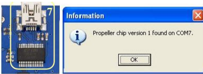
Figure 2.8 The USB connector and FTDI 232RL chip successfully detected the microcontroller.
