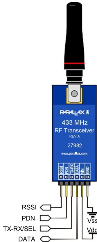
Figure 4.4 Wireless communication using 433 MHz Transceiver.
