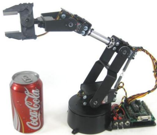
Figure 1.4 4 DOF Manipulator / arm robot from Lynxmotion suitable for education (source: lynxmotion.com).
