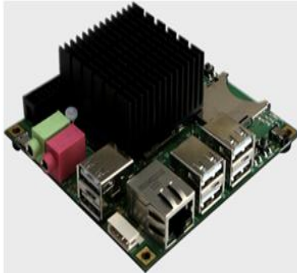
Figure 10.2 Odroid X2 for processing the images from webcam ( hardkernel.com, 2013 ).
